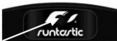
switches between the coded channels. If you press and hold the button for 5 seconds, it will automatically switch to the uncoded channel. Pressing the button again will switch back to the encoded channels.
